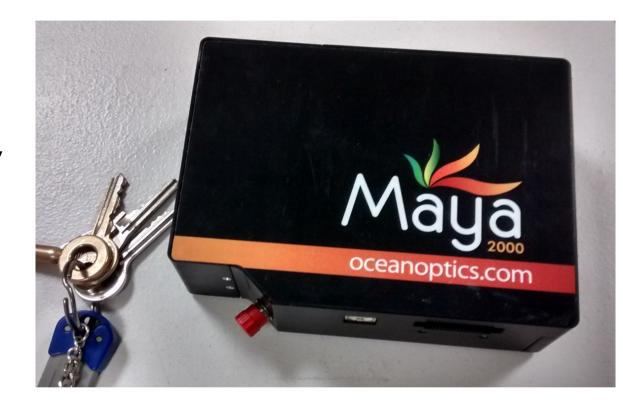
MayaPRO is in the high-end of the Ocean Optics visible spectrometer range. It is more sensitive and the sensitivity extends up to 1050 nm in the near-infrared.
