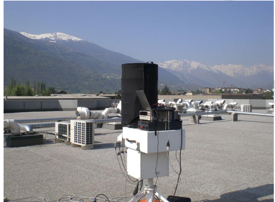
1000W “portable” calibrator for Brewer in Aosta, Italy
