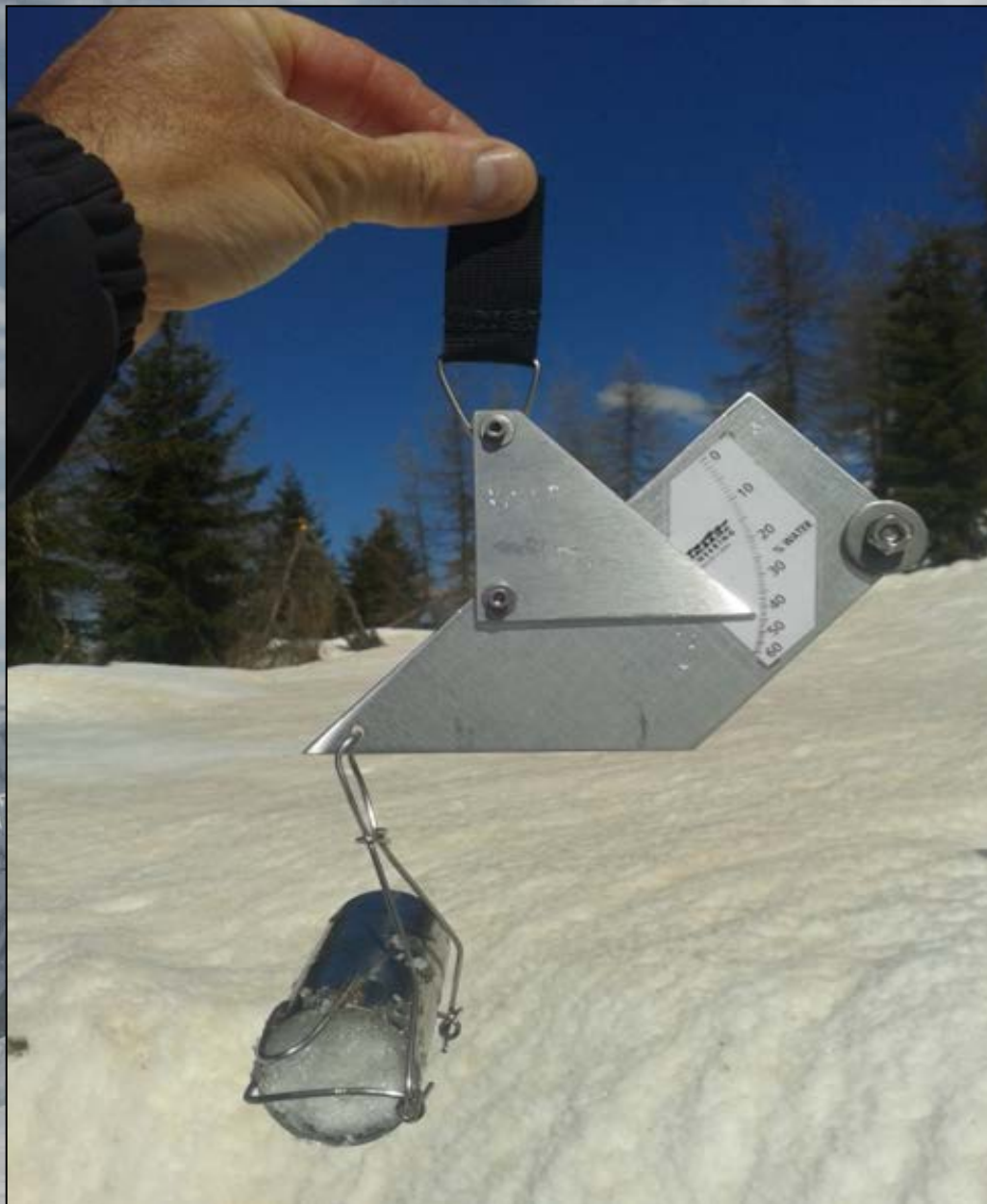
Example of snow weight directly using the snow sampler
