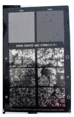
Figure 4. Magnifier (left) and crystal card (right).
