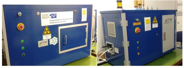
Figure 11. Two Computer tomographs in the cold lab. µCT80 (left), µCT40 (right)
