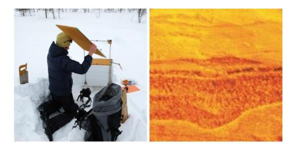
Figure 5: Preparing to take an NIR photograph of a snow profile (left). Image of a snow profile captured by NIP (right). The picture clearly reveals the individual layers, even if they are very thin.
