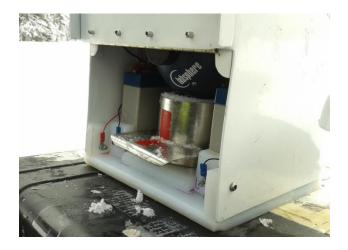
Figure 8. Extracted sample for IRIS measurement (left) Sample is placed inside IRIS under the sphere
