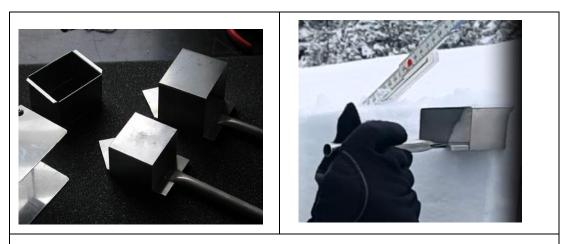
Figure 2. Density cutter (left) inserted into the snow layer (right)
