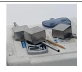
Figure 3. Excess snow is cutted with the lid (left) DC fulled with snow is weighed by digital scale
