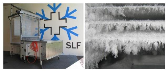
Figure 10.: SnowMaker (left) and nature-identical dendritic snow on the cultivating threads (right).
