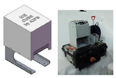
Figure 7. Laser reflectometer devices. IceCube (right) IRIS (left)
