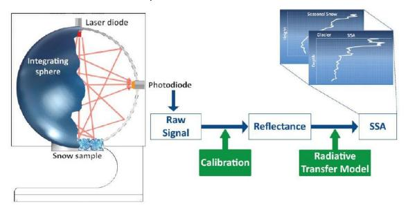
Figure 6. Working principle of laser reflectometer
