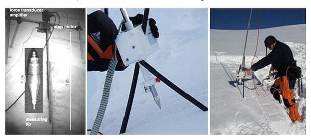
Figure 9. Measuring tip at the end of the rod (left) Motor unit, black poles and the tip (middle) measurement by an SMP (right)
