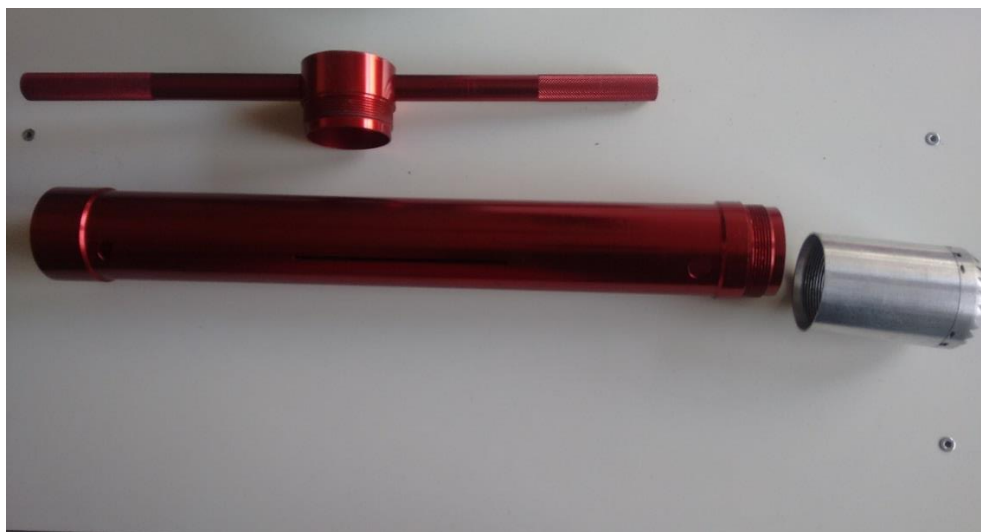
Figure A8. Composition of the snow tube. In the picture, there is only one of the total 6 elements of the tube.
