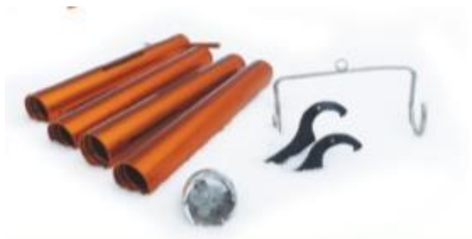
Figure A11. The Enel-Valtecne EV2 snow tube. From left: 4 elements of the tube, the drilling tip, the support for the weighing and the two wrenches for disassembling the tube after drilling operations
