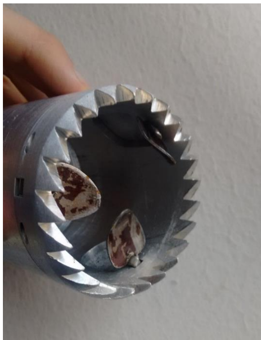
Figure A9. Detail of the drilling tip of the snow tube.
