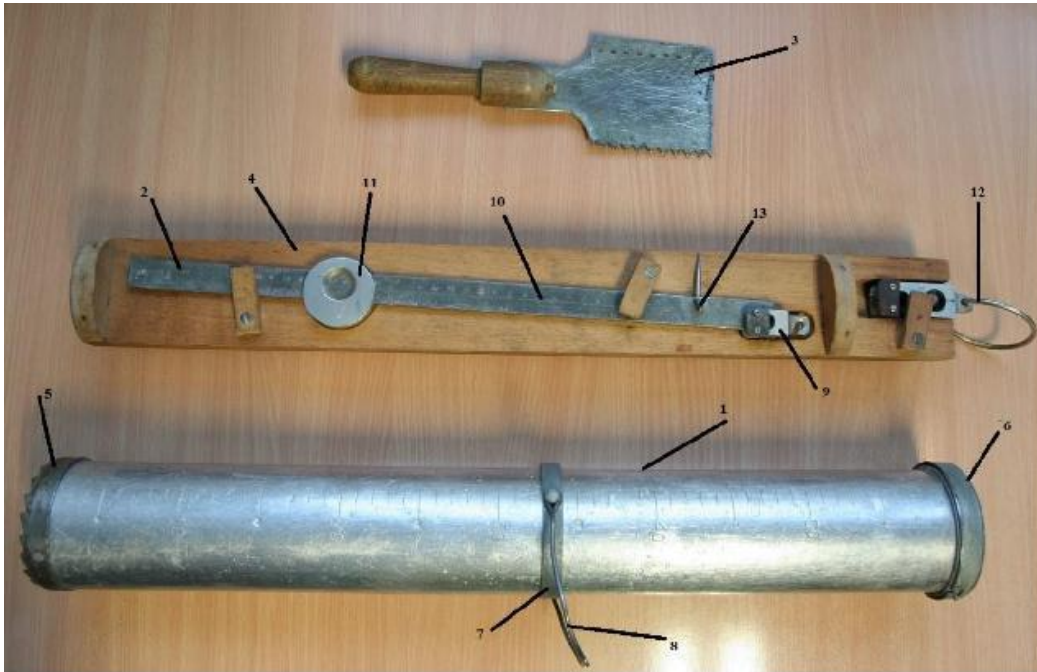
Figure A1. SWE tube VS-43. 1 – cylinder; 2 – scale; 3 – a sharp shovel; 4 – wooden base; 5 – a sharp ring; 6 – cover of cylinder; 7 – hoop; 8 – handle; 9 – hook of scale; 10 – scale bar; 11 – left; 12 – handle.
