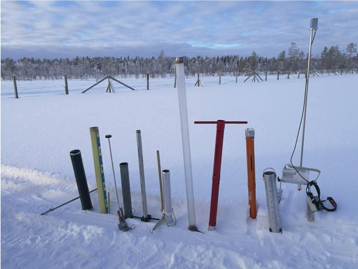
Figure 1. The instruments used in the 3 rd HarmoSnow field campaign (from left to right): Korhonen-Melander (made and used in Finland), Dolfi (used in Slovakia and Czech Republic; made in Czech Republic), VS-43 (used in Estonia; made in Russia), U.S. Federal (used in Turkey; made in USA), IG PAS (made and used in Poland), SnowHydro (used in Spain; made in USA), Custom EV2 (made and used in Italy), Enel-Valtecne EV2 (made and used in Italy) and ETH (made and used in Switzerland and Spain). In addition, the SnowMicroPen (made in Switzerland) is shown on the far right side.
