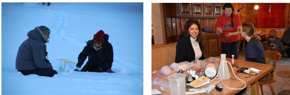
Figure 3: Sampling of surface snow for EC/OC analysis (right) and filtering of samples (left)
