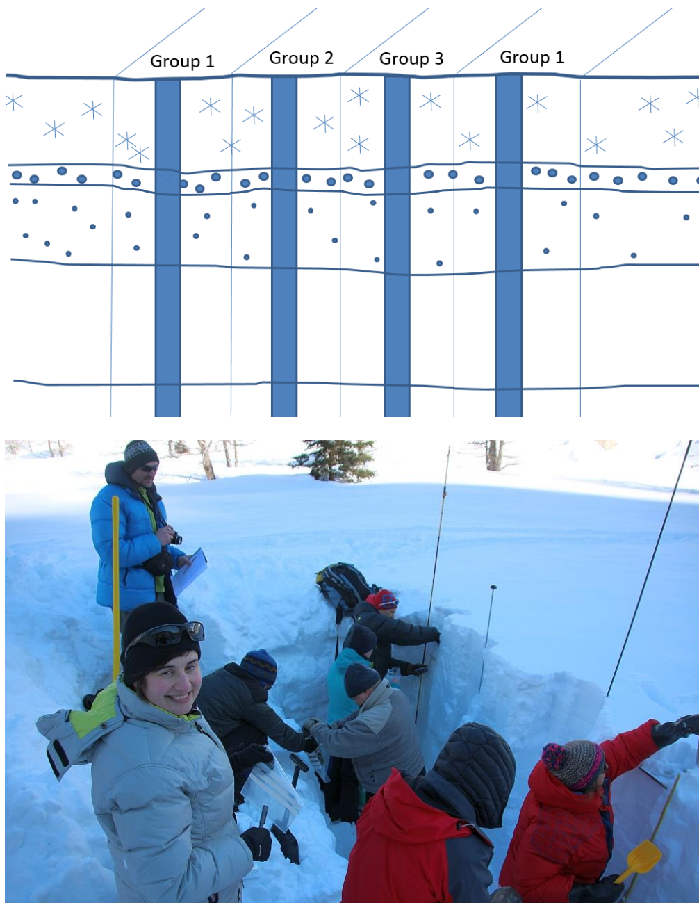
Figure 1: The general concept and realization of the snow sampling inter-comparison experiment at Sonnblickbasis (from the left to the right: Team Austria1, Team Poland, Team Italy, Team Austria2 and to the right (not shown in the photograph) the location of second sampling of Team Austria 1 again).
